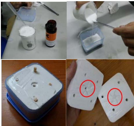
Fig. 5 Creation of silicon mold for wax injection
