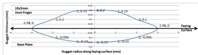
Fig. 8 Nugget geometry of 10x5mm vent finger
