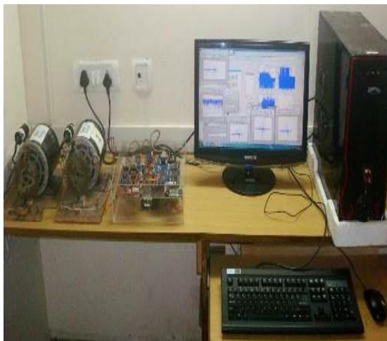
Fig. 3 Experimental setup using healthy and unhealthy motor
