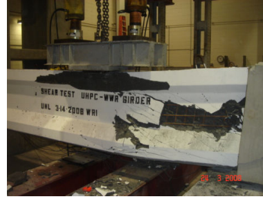
Fig. 8 Girder test (limit state)
