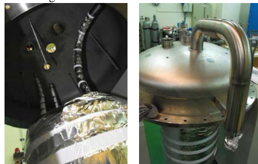
Fig. 2 The nitrogen vessel is covered with multiple super-insulation layers and then hung to the cover of the vacuum shielding vessel
