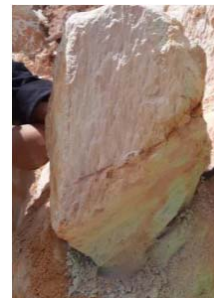
Fig. 4 Block sample of uncemented sandstone
