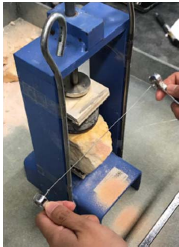
Fig. 5 Uncemented sandstone trimming process
