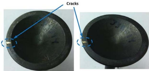
Fig. 2 Cracks at the "blade" area after coining
