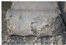
Fig. 6 Decomposition of a specimen exposed to 900°C
