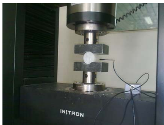
Fig. 2 Servo-electric loading frame with AE monitoring system
