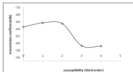
Fig. 7 Transmission coefficient of a nonlinear PhC lattice as a function of the nonlinearity.
