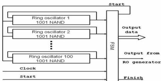
Fig. 8 Array of ring oscillator with same length
