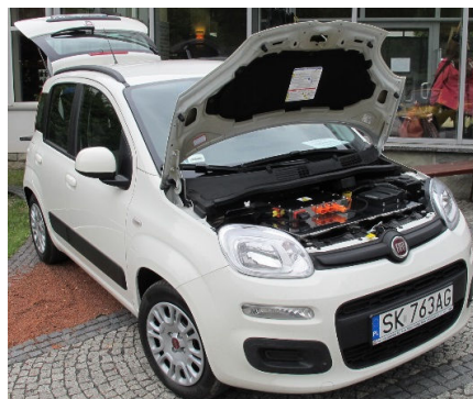
Fig. 1 Fiat Panda with Komel's PM motor – research and development project no. NR01-0084-10
