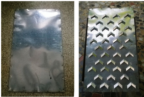
Fig. 3 Smooth and roughened absorber plate
