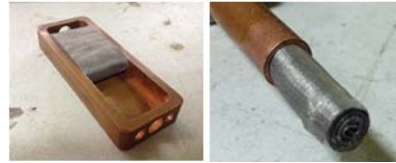
Fig. 4 Stainless steel screen mesh capillary wick
