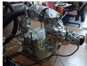
Fig. 6 Flat plate loop heat pipe assembly.
