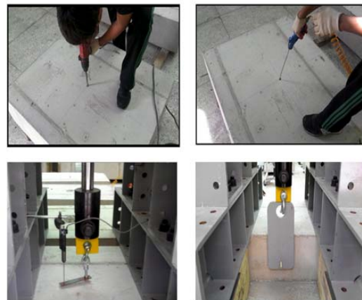
Fig. 4 Test Setup for Post-Installed Anchor Systems
