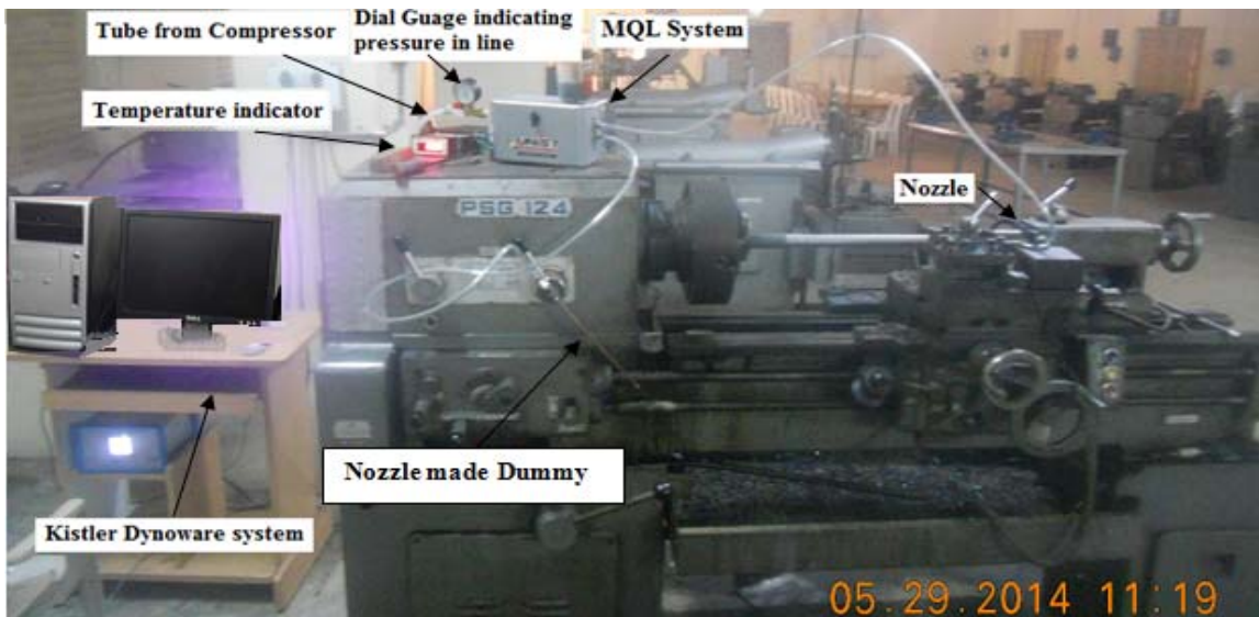
Fig. 1 Experimental set up with Coolubricator system
