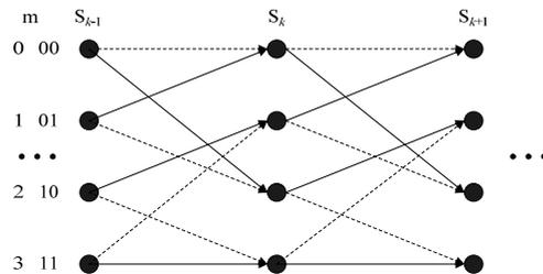
Fig. 4 Trellis diagram of the RSC code
