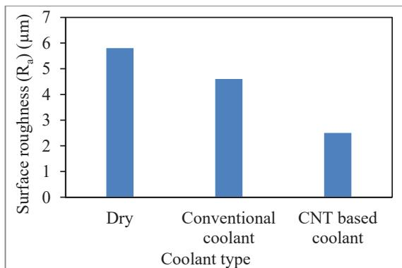
Fig. 8 Surface roughness under different coolant conditions
