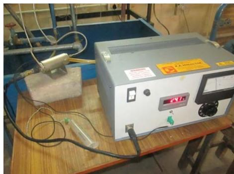
Fig. 3 Thermal conductivity apparatus
