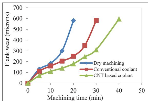
Fig. 7 Flank wear at different lubricating conditions
