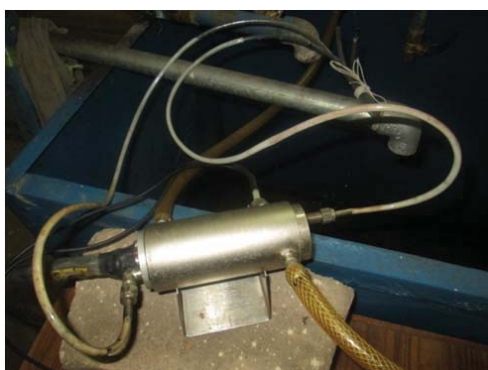
Fig. 4 Magnified view of plug and jacket assembly
