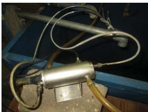
Fig. 4 Magnified view of plug and jacket assembly
