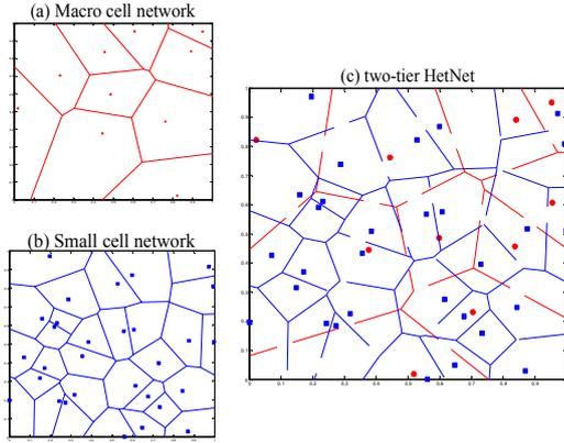
Fig. 1 Voronoi tessellation of two-tier Heterogeneous Networks
