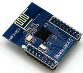
Fig. 7 Minimum working development BLE module nRF51822 SoC
