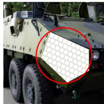
Fig. 2 Ceramic composite armor used for military vehicles [10]
