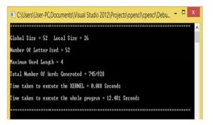
Fig. 2 (c) Time taken by the Kernel and the whole program with Work Item size = 26 and Work Group size = 2
