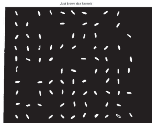
Fig. 8 Paddy and rice kernels at various stages of image processing (a) Noise removed, (b) b/r ratio, (c) Binary image of b/r, (d) Just brown rice kernels
