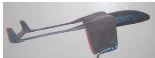
Fig. 3 UAV with a down-horizontal stabilizer and without landing gear
