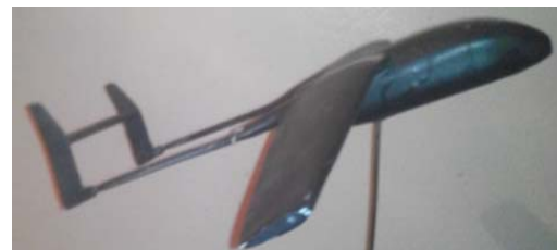
Fig. 2 UAV with an up-horizontal stabilizer and without landing gear
