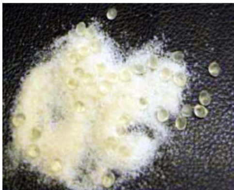
Fig. 3 Example of newer mixed-size particulate diverter
