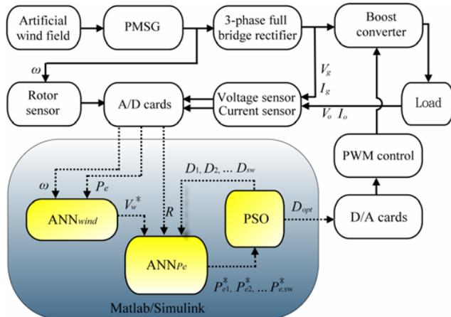
Fig. 5. Block diagram of the MPPT control Process.
