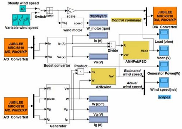
Fig. 6. Simulink structure of MPPT control.
