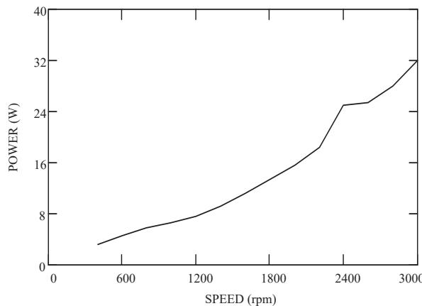
Fig. 2 Mechanical losses of the induction motor
