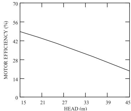
Fig. 11 Motor efficiency
