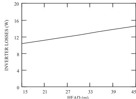
Fig. 6 Inverter losses
