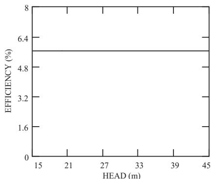
Fig. 3 Array efficiency at constant reference insolation
