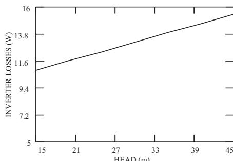
Fig. 8 Inverter losses
