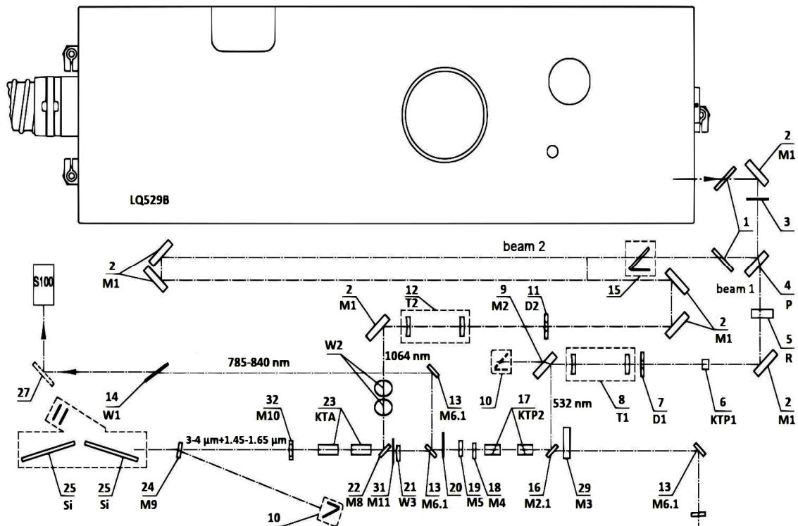
Fig. 1 Optical diagram of the laser system
