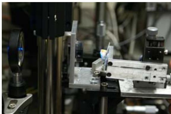
Fig. 9. OCT Fluorescence investigation in order to detect the micro leakage of the resin filling for sample 79.
