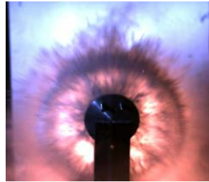
Fig. 8 The shape of liquid dispersion flow, when the detonation cord is 5\text{ g} \cdot \text{m}^{-1} , the diameter of cylindrical film is 150mm. The liquid is the mixture of water and glycerin with capacity ratio of 5:5
