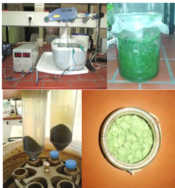
Fig. 3 Microalgae harvesting, desalinating and drying
