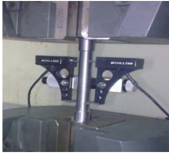
Fig. 2 Extensometer set on the plain specimen during the tension test
