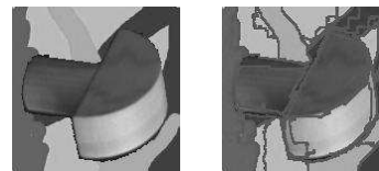
Fig. 9. A view of an object is firstly rotated and rescaled, then displayed on a cluttered background (on left) and finally it is segmented (on right) in order to extract the number of regions composing the transformed segmented object view.
