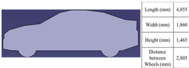
Fig. 2 Specifications of the vehicle of this simulation
