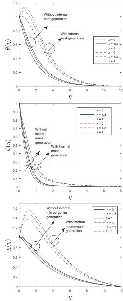
Fig. 3 Profiles of  $f'(\eta)$   $\theta(\eta)$   $\phi(\eta)$   $\chi(\eta)$  for various values of  $\lambda$
