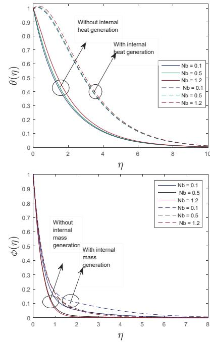
Fig. 6 Profiles of  $\theta(\eta)$  and  $\phi(\eta)$  for various values of  $Nb$   $\gamma = 0.05$ ,  $Nt = 0.1$ ,  $Le = 5$ ,  $Lb = 0.5$ ,  $Pe = 0.3$ ,  $\sigma = 0.2$ ,  $\lambda = 1/3$ ,  $c = 0.1$ ,  $M = 0.5$ ,  $Pr = 0.71$
