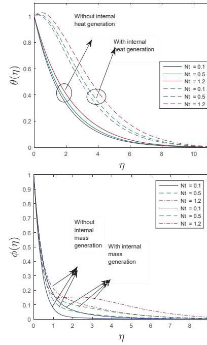
Fig. 5 Profiles of  $\theta(\eta)$  and  $\phi(\eta)$  for different values of  $Nt$   $\gamma = 0.05$ ,  $Nb = 0.5$ ,  $Le = 5$ ,  $Lb = 0.5$ ,  $Pe = 0.3$ ,  $\sigma = 0.2$ ,  $\lambda = 1/3$ ,  $c = 0.1$ ,  $M = 0.5$ ,  $Pr = 0.71$
