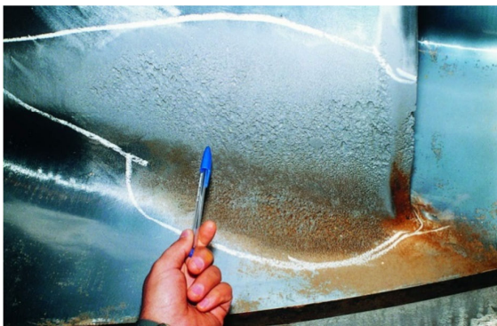
Fig. 1 Cavitation damage on runner blade surface
