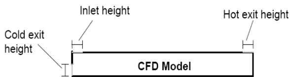
Fig. 2 Schematic of the computational domain.
