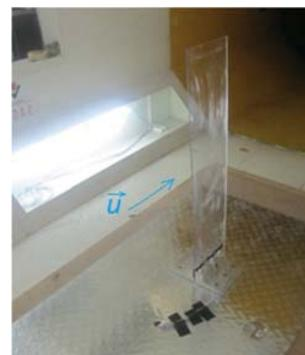
Fig. 2 Experimental setup for PC plate structure in Wind tunnel,
