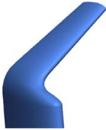
Fig. 11: Geometry of the first analyzed winglet
