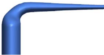
Fig. 14: Geometry of the second analyzed winglet
