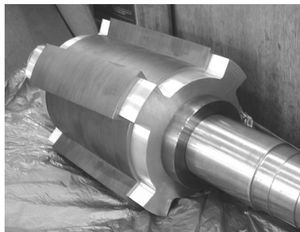
Fig. 14 Skewed rotor of 6-phase RDCM
