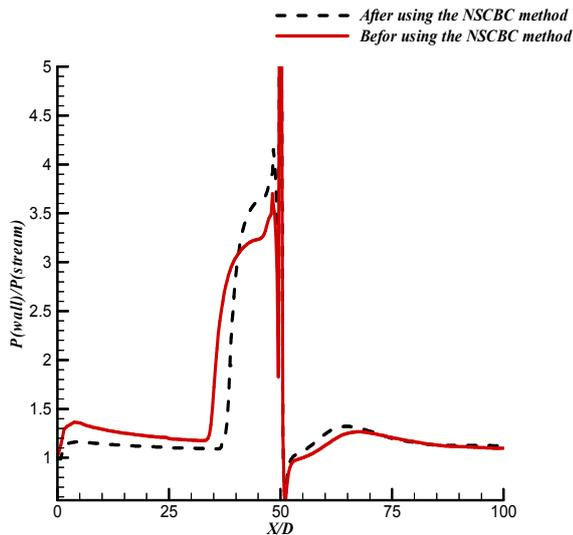
Fig. 2 Pressure profiles on the wall
