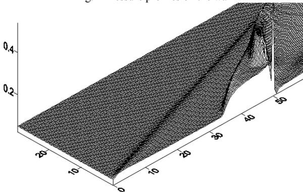
Fig. 3 Pressure distribution before applying the NSCBC method
