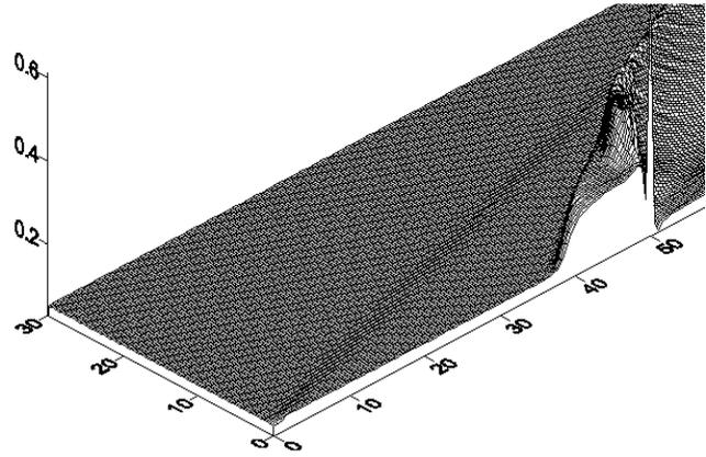
Fig. 4 Pressure distribution after applying the NSCBC method
