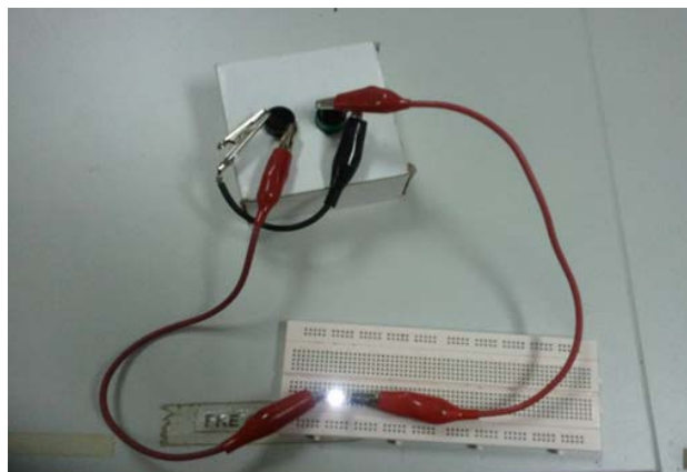
Fig. 5 Two series of compacted vermicompost can light up LED
