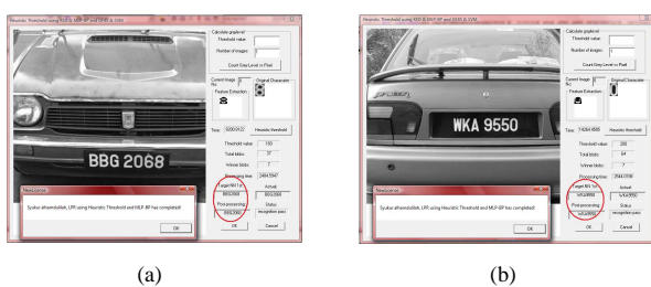
Fig. 9. Successful image results based on Heuristic Threshold, and MLP-BP classification techniques.
