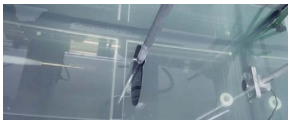
Fig. 3 Picture of the experimental set-up where hydrophone, FZP and piston transducer are shown
