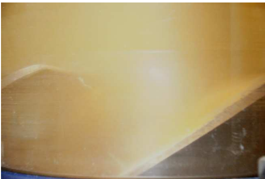
Fig. 15 Cavitation pattern under operating condition of No. 3-5
