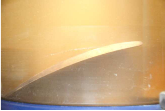
Fig. 7 Cavitation pattern under operating condition of No. 2-2
