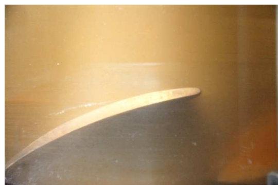
Fig. 6 Cavitation pattern under operating condition of No. 2-1
