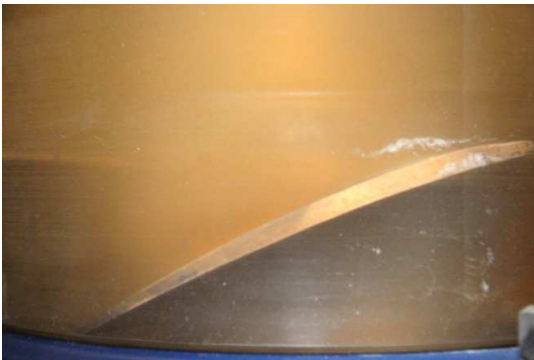
Fig. 8 Cavitation pattern under operating condition of No. 2-3
