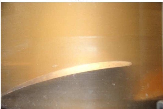
Fig. 3 Cavitation pattern under operating condition of No. 1-3
