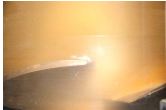
Fig. 5 Cavitation pattern under operating condition of No. 1-5
