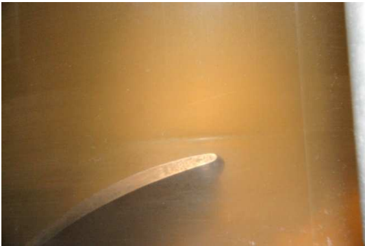
Fig. 14 Cavitation pattern under operating condition of No. 3-4
