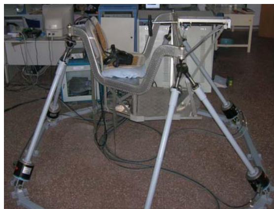
Fig. 1 The parallel motion platform with subsided cabin
