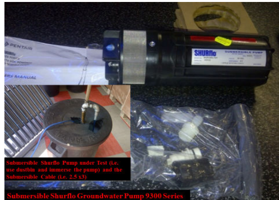
Fig. 7 Solar Groundwater Submersible Pump and under test
