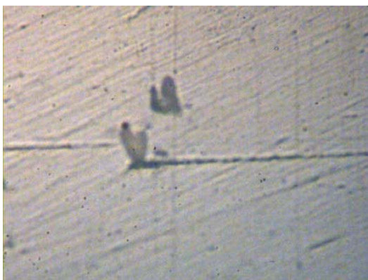
Fig. 17 Specimen with crack angle of 90° with crack depth of 4mm that was fractured at strain rate 1.43 \times 10^{-3} \text{ s}^{-1}
