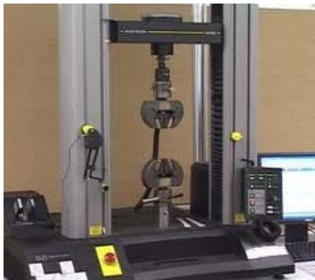
Fig. 2 A model 3369 Instron Universal Tensile Testing Machine
