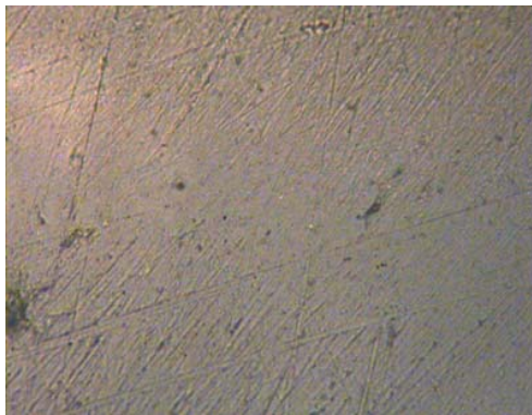
Fig. 15 Plastic region of specimen with crack depth of 2mm at crack angle of 90° that was fractured at strain rate 0.95 \times 10^{-3} \text{ s}^{-1}
