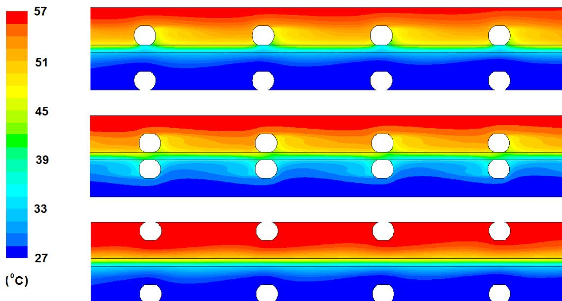
Fig. 2 Temperature profiles in spacer-filled channels
