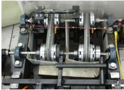
Fig. 6 Prototype of DBCVT and test rig
